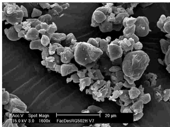
Fig. 4. SEM of placebo microparticles made of Resomer® RG 502H after preparation as described in Table 2 run 7.
